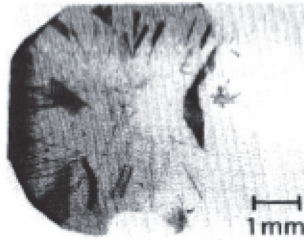
Figure 3: 2-D X-ray topography of IIa HPHT diamond showing stacking faults (black areas) (from H Sumiya et al, “Crystalline Perfection of High Purity Synthetic Diamond Crystal” (1997) 178 Journal of Crystal Growth 485 at 490)
