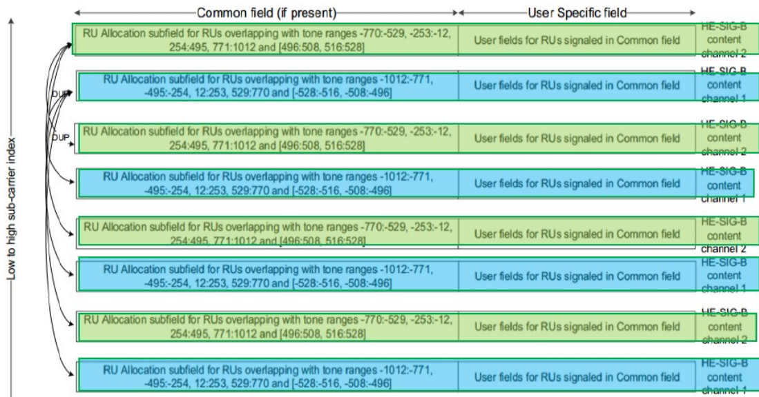
Figure 27-31—HE-SIG-B content channels and their duplication in a 160 MHz PPDU
